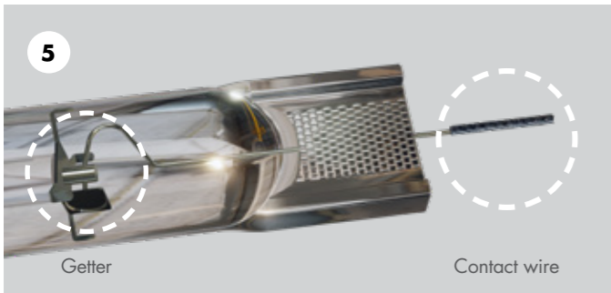
Before placing the new lamp, make sure the contact wire is straight, the getter is on the ballast side and the text on the lamp is facing out.
