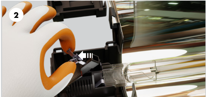
Slide both fittings fully open, as shown
